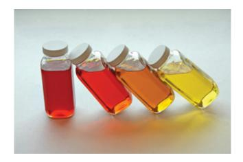
A Sample of CDSO on left, and biodiesel produced by various technologies - *Bob Modersohn*
