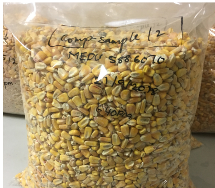
Figure 7. Example of reference sample of U.S. corn taken from a composite sample during container unloading.
