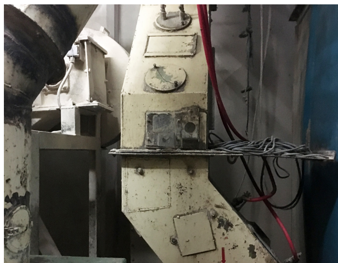
Figure 9. Mold inhibitor application system located in the grain receiving system at the Malaysian facility.
