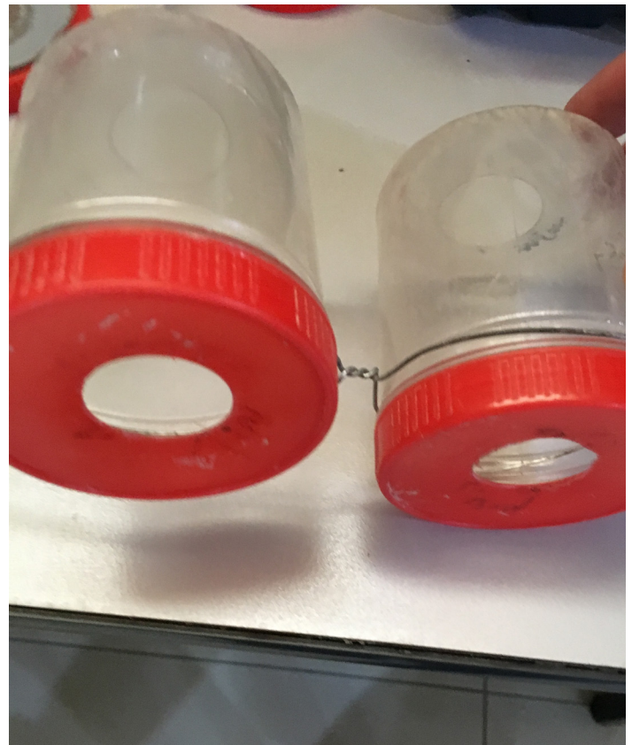
Figure 12. Example of plastic containers (with a hole on the lid covered with a mesh) used as insect bioassays.
