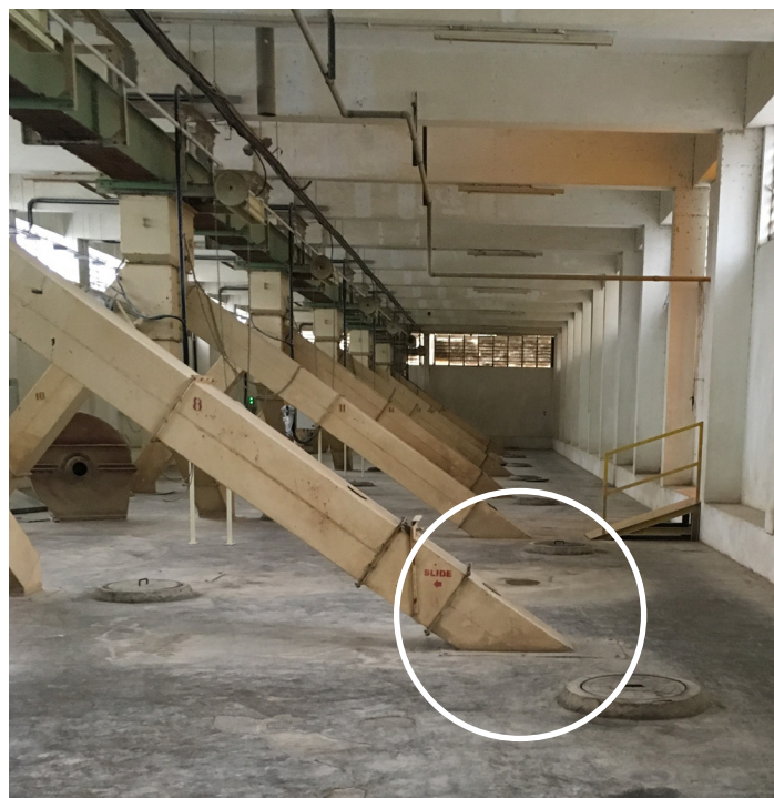
Figure 11. Example of the sampling port (shown in circle) at the top of the concrete silos used for each of the grain quality management strategies.
