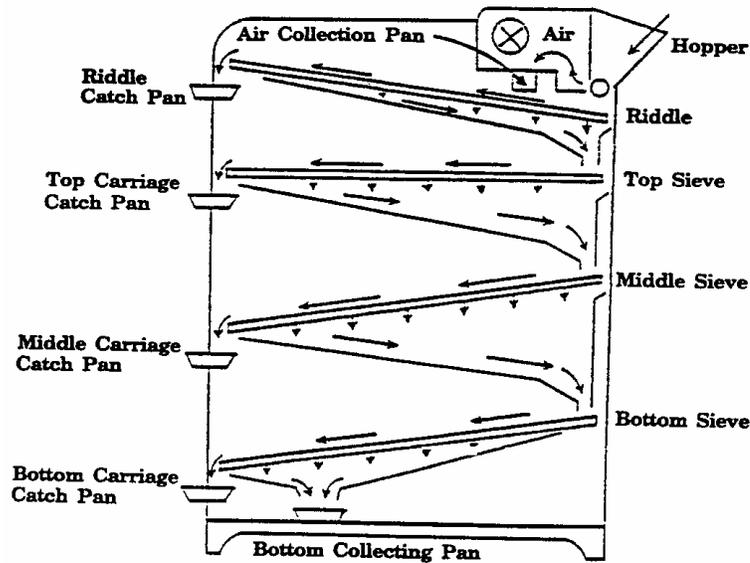
The Dockage Tester also is used to determine the percentage of broken corn and foreign material in corn. Broken corn and foreign material is a grading factor in corn.
