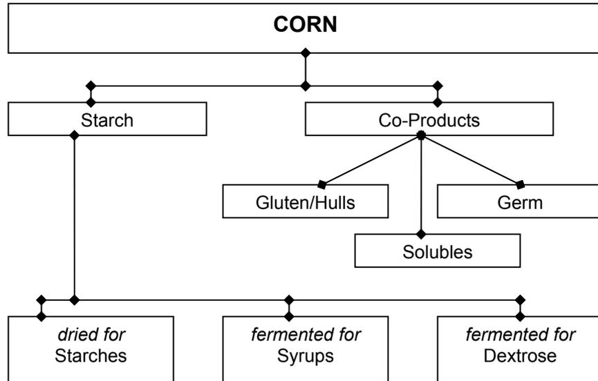
The most promising areas of new research and opportunity for industrial uses lie in expanding the use of feed grains as a substitute for petroleum. There is no molecular hydrocarbon derived from petroleum that cannot be replicated from the starch feedstock.
